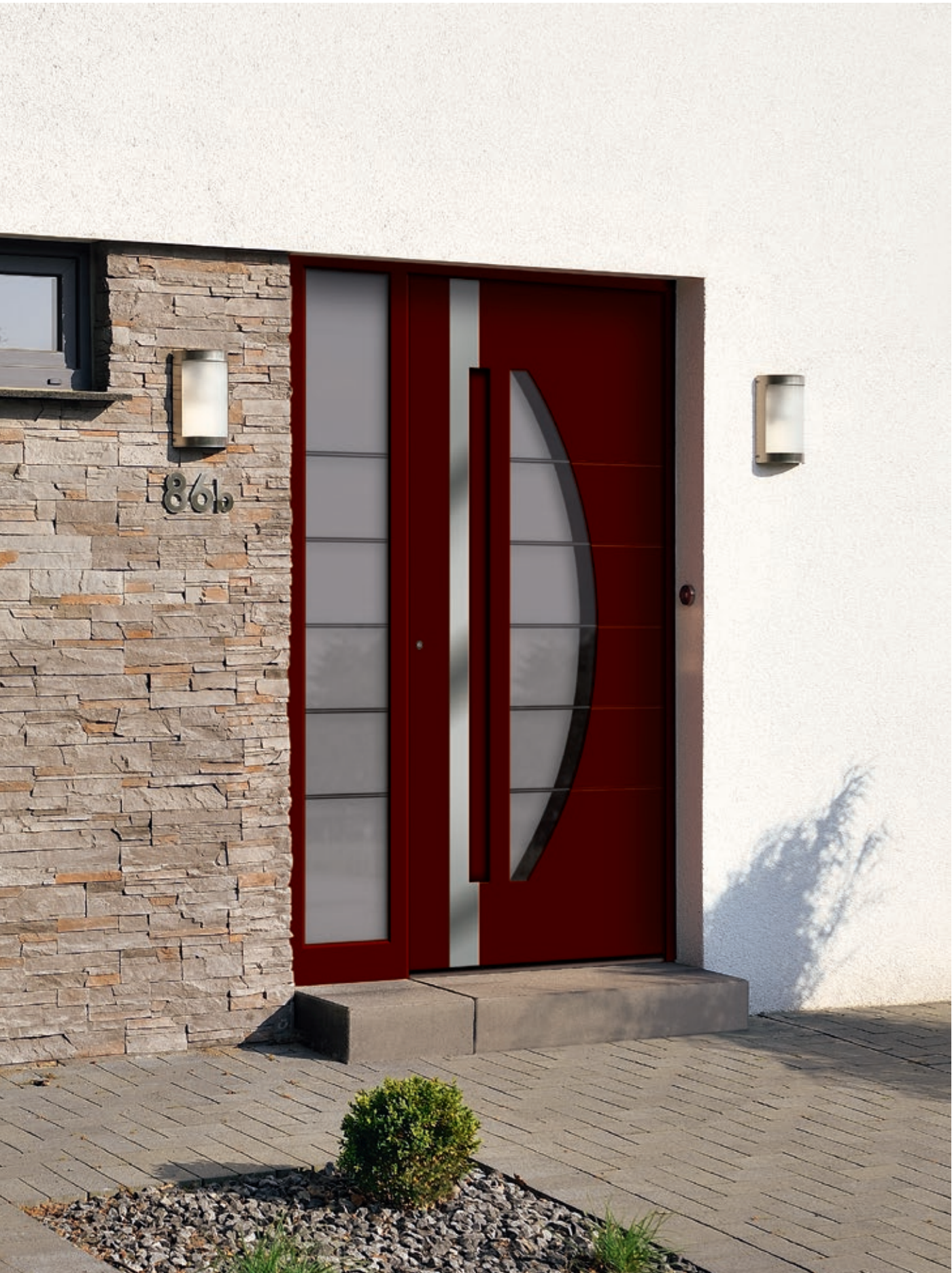
Model 6973-41 with all glass side panel | application – stainless steel flush | integrated handle element | sash overlapping panel | glass: G 1168 frosted glass with edge stripes and clear stripes | extras: RAL 3005 vine red | Only available as sash overlapping door panel! Optionally available with LED-Lighting 6973-44.
